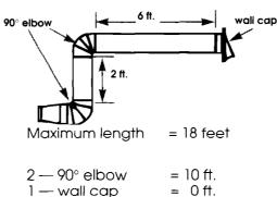
$1 - 90^{\circ}$  elbow = 10 ft. 1 - wall cap = 0 ft. 8 feet straight = 8 ft.Length of 6" system = 18 ft.
